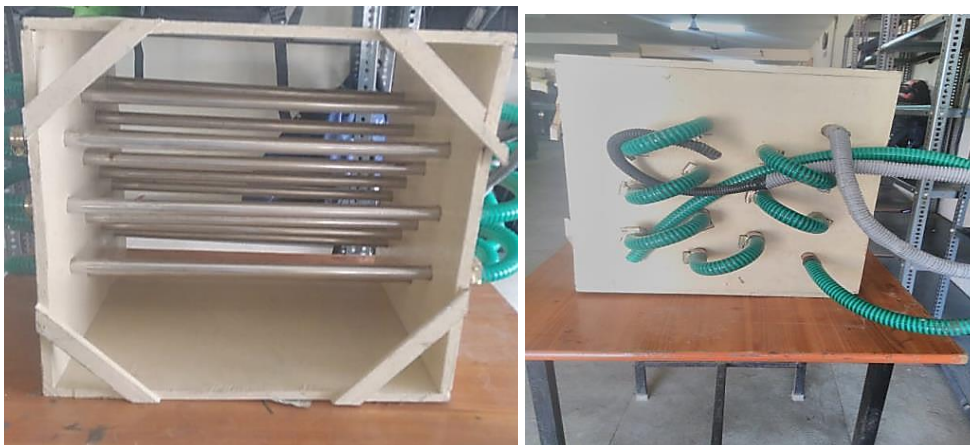
Air Cooled Heat Exchanger Test setup
